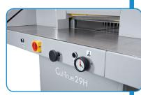
Two-button operation, fine-tune knob, adjustable hydraulic pressure gauge
