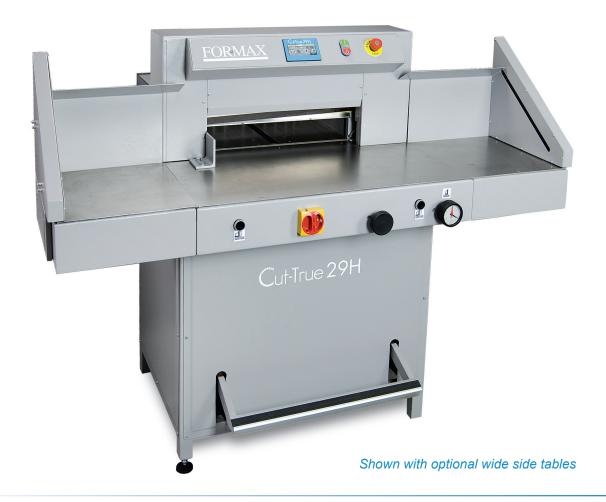
The Formax Cut-True 29H Hydraulic Guillotine Paper Cutter offers precision cutting for paper stacks up to 20.5" wide. User-friendly, intuitive features include a touchscreen control panel, automatically-adjusting back gauge and the capacity to program up to 100 jobs/100 cuts. An infrared light beam safety curtain provides safety and convenience as it shuts down operation if the light plane is interrupted.
